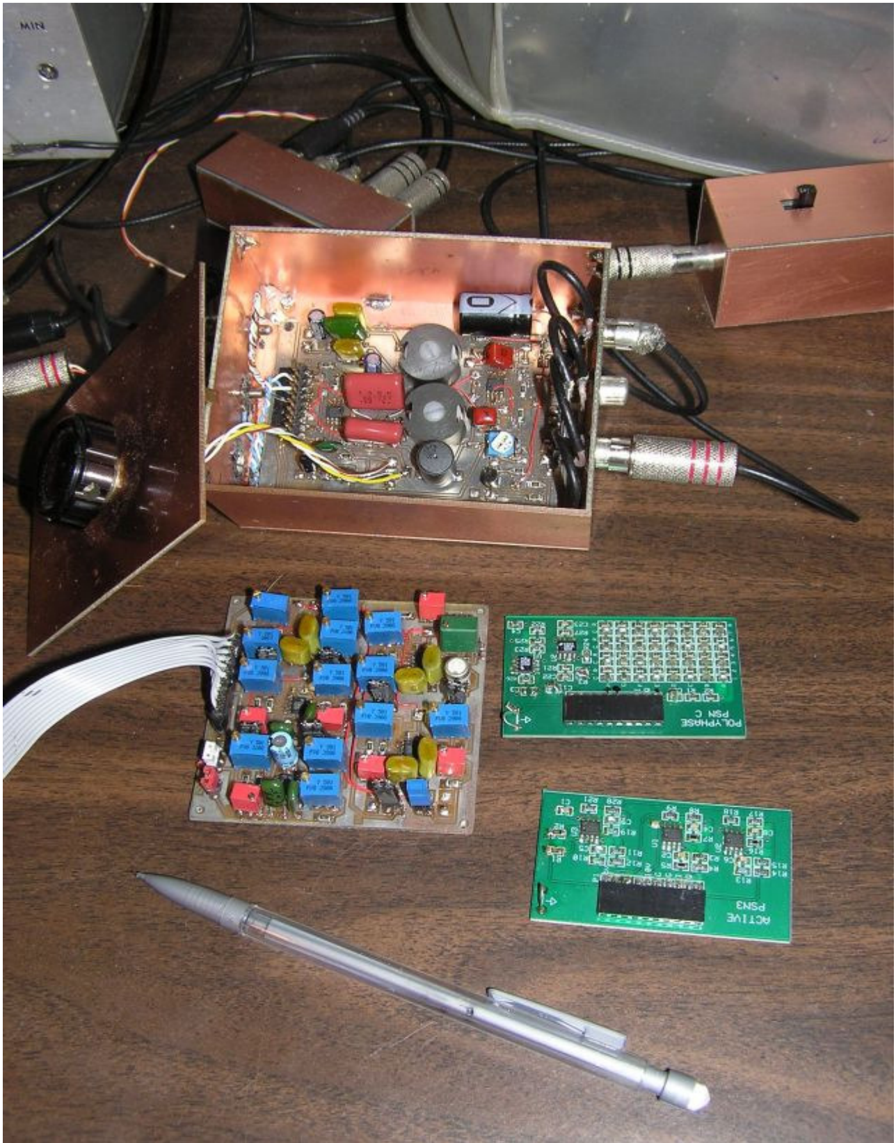
W6JL Receiver's Phasing Section, with three plug-in phasing boards.
