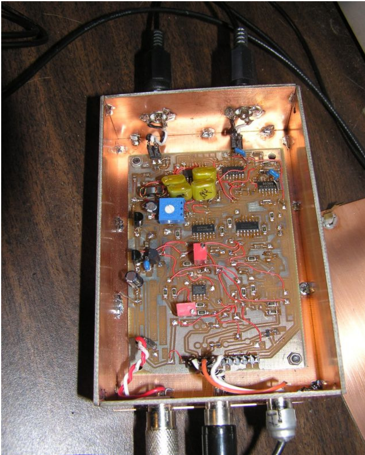
My third Tayloe (Q.S.D.) front end for W6JL Receiver, built on a homebrew PC board. Parts deleted are for selectable sideband, which are not needed for CW-only ops like myself. This further simplifies an already simple front end.
